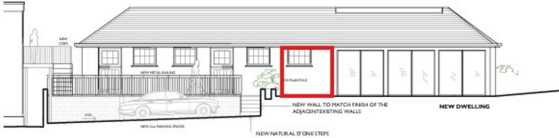
Proposed Front Elevation indicating infill panel.
