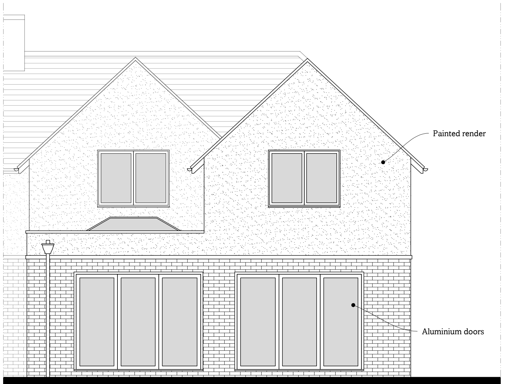
Existing East Elevation 1:50
