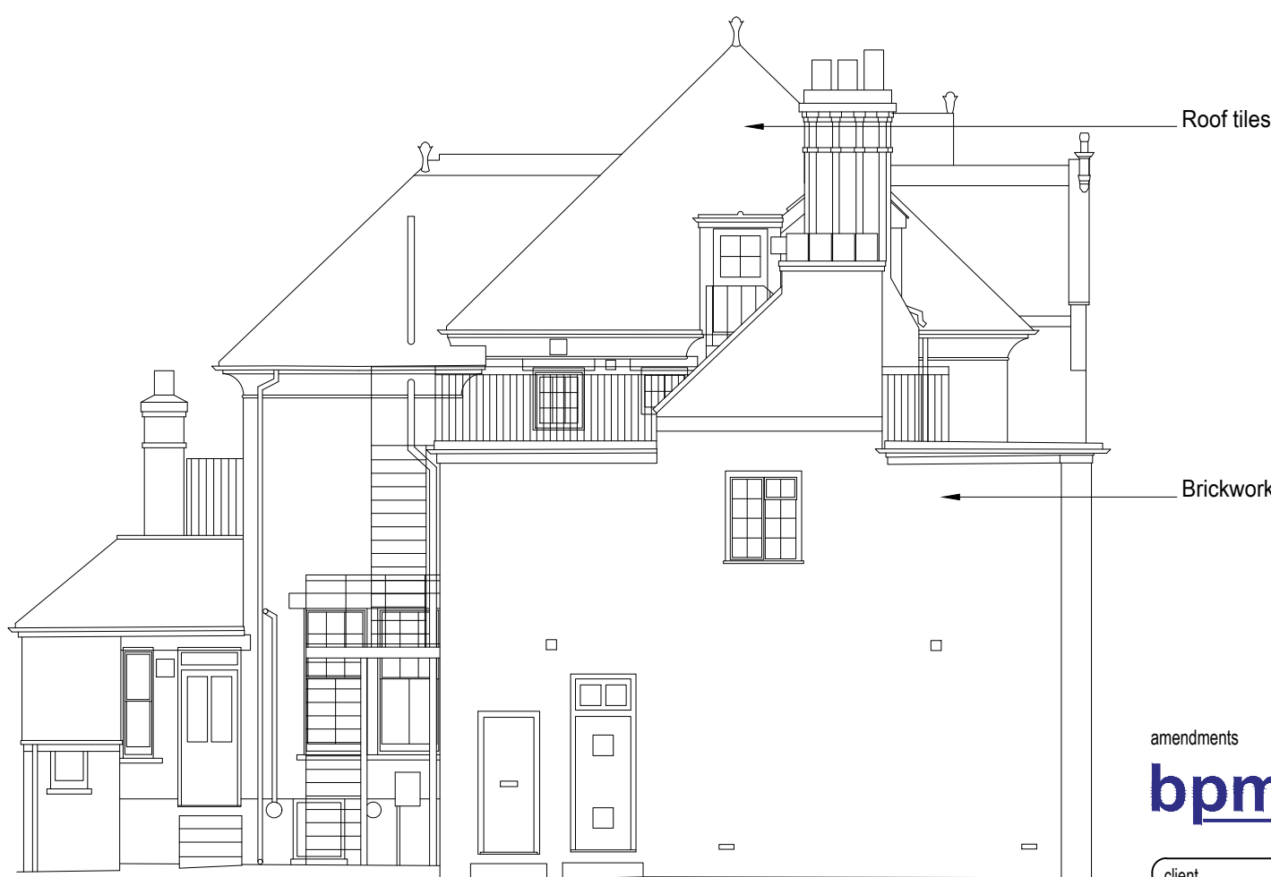
Existing Side Elevation (North) 1:100
