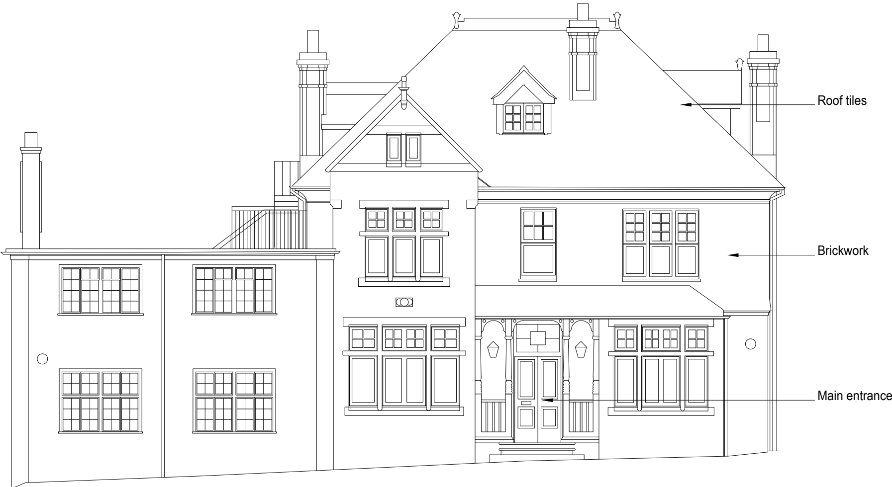
Existing Front Elevation (West) 1:100
