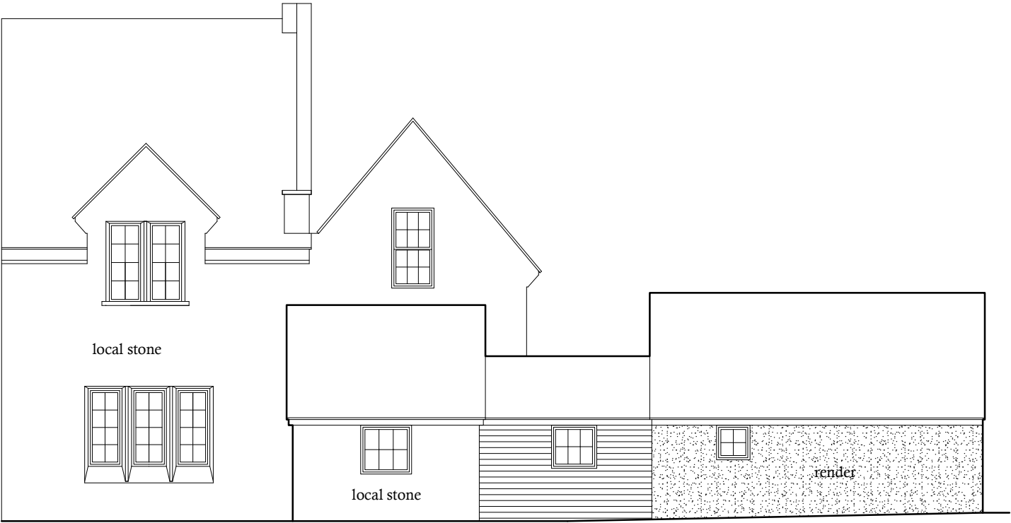
EXISTING REAR ELEVATION Facing East
