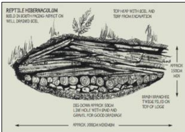
Figure 20. Illustration on how to build a reptile hibernaculum. Image produced by ARG UK.
