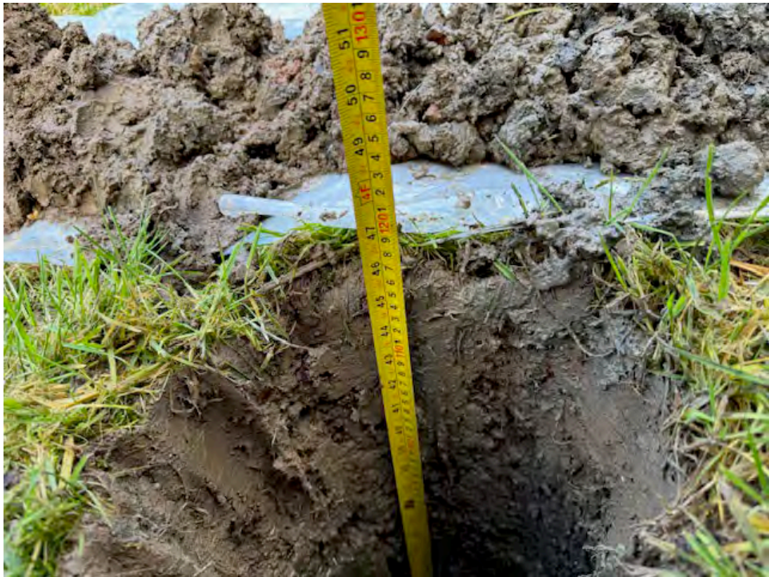
TP1 depth upon completion
