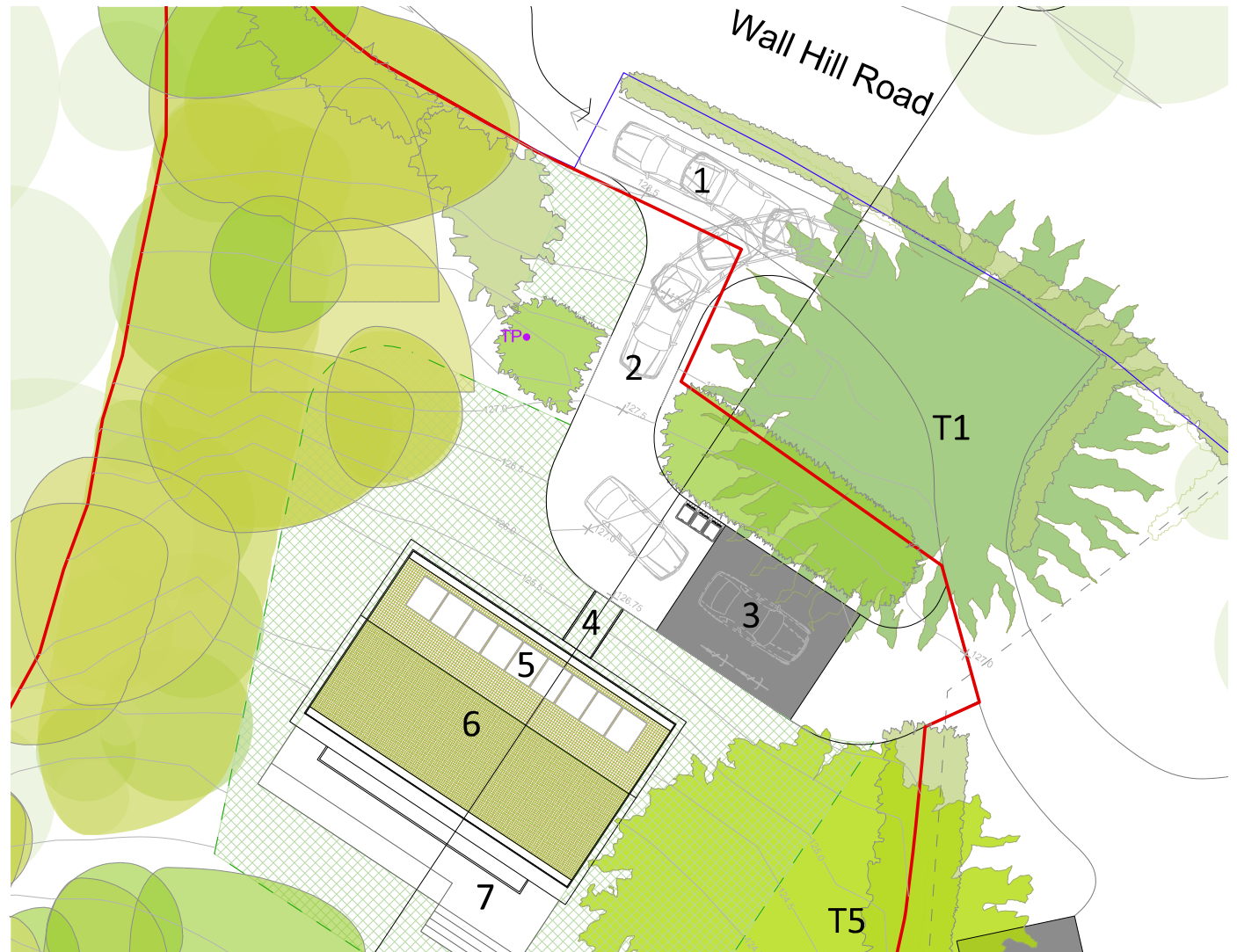
Proposed site plan showing the single drive-through garage located behind the existing hedge
