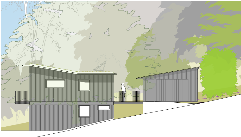
Proposed east elevation showing single garage with a lower roof profile and level entry bridge
