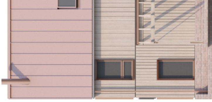
Eave and window detail, down pipe and timber cladding.
