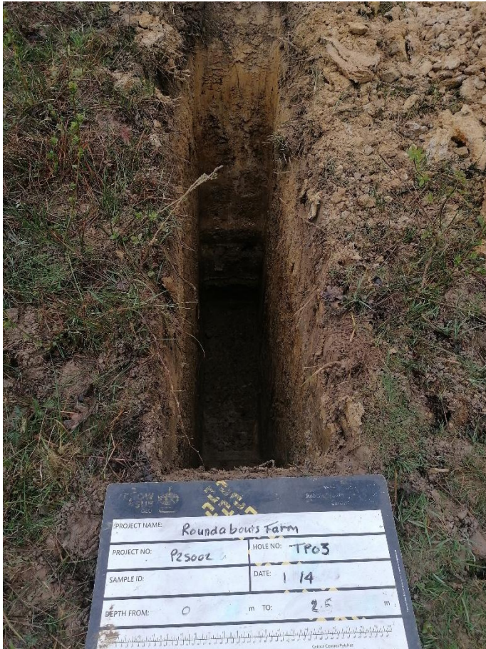
TP03 trial pit
