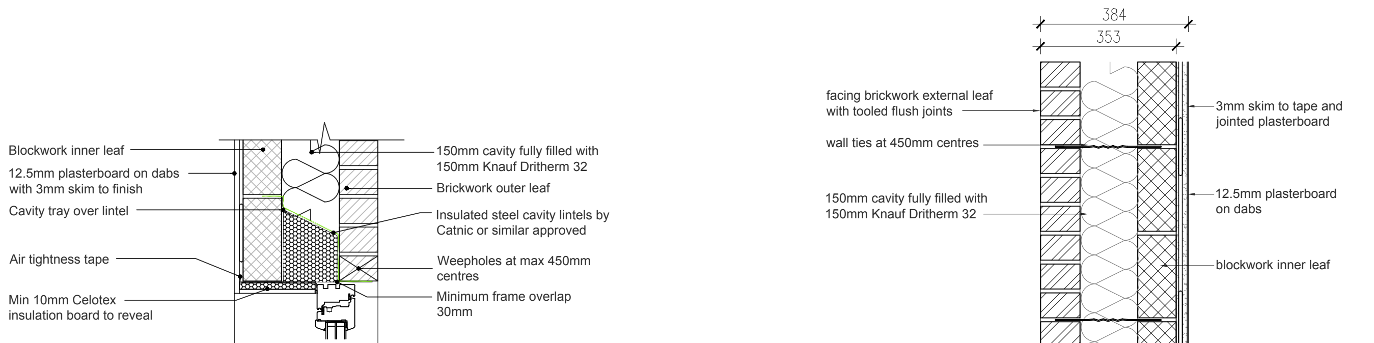
Detail 3-3 External wall / window head detail 1:10
