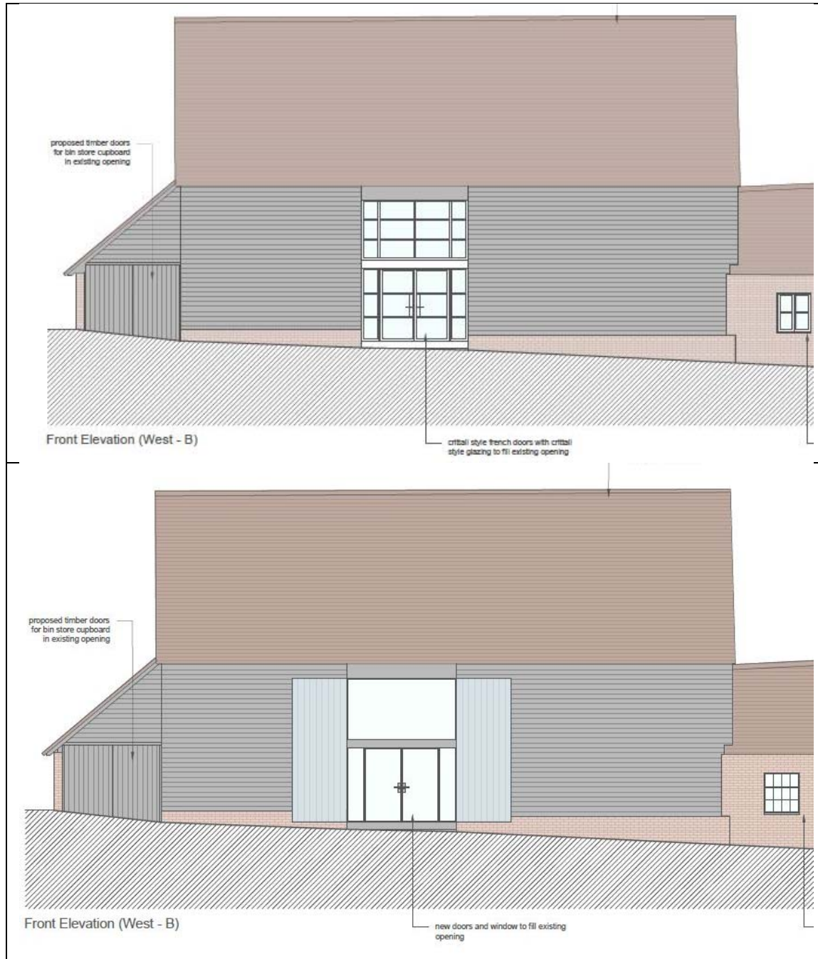
Plate 8: The original glazing scheme (top) and the revised scheme (bottom)
