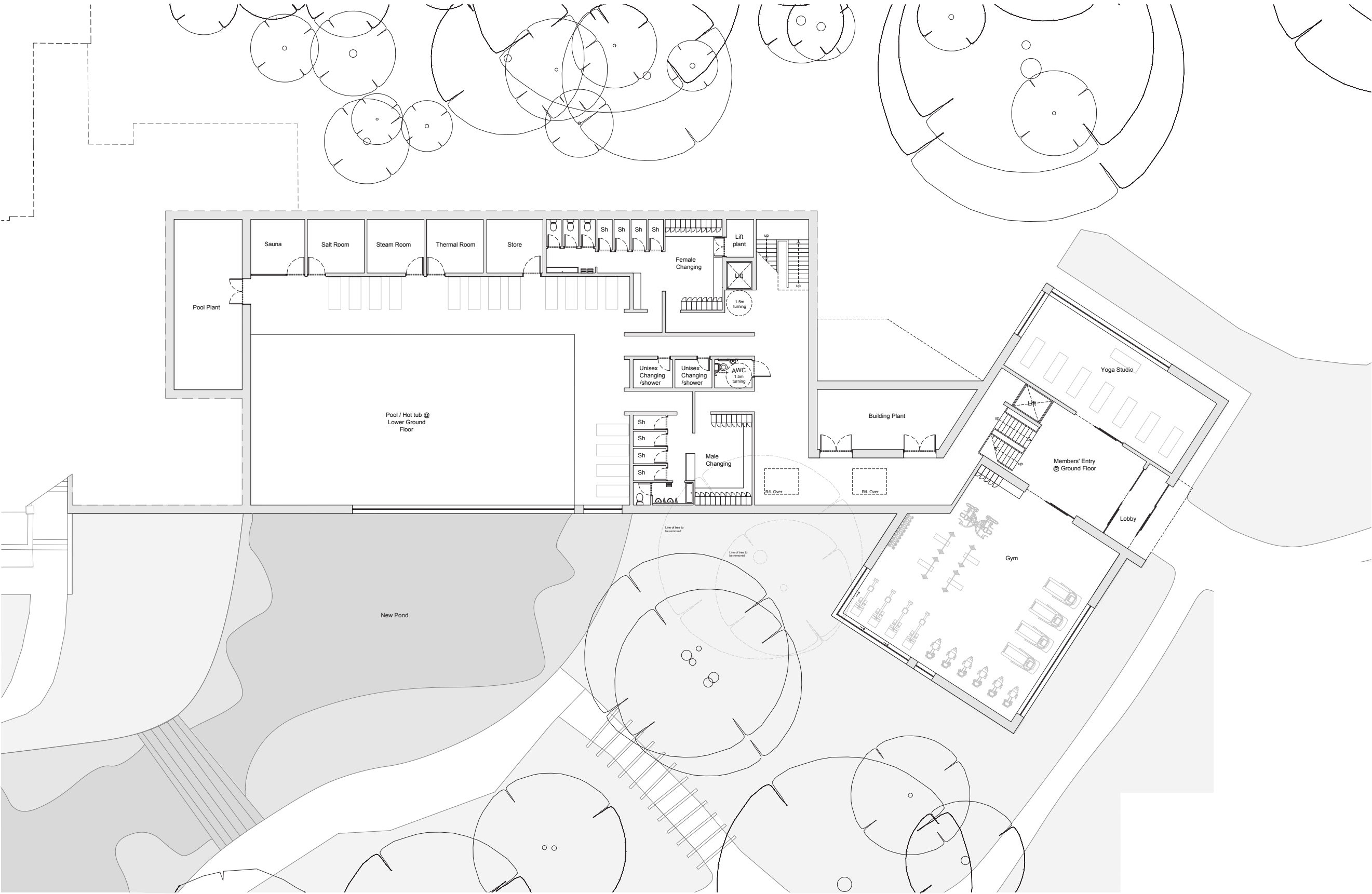
Lower Ground Floor Plan (pool) + Ground Floor Plan (gym & yoga studio)
