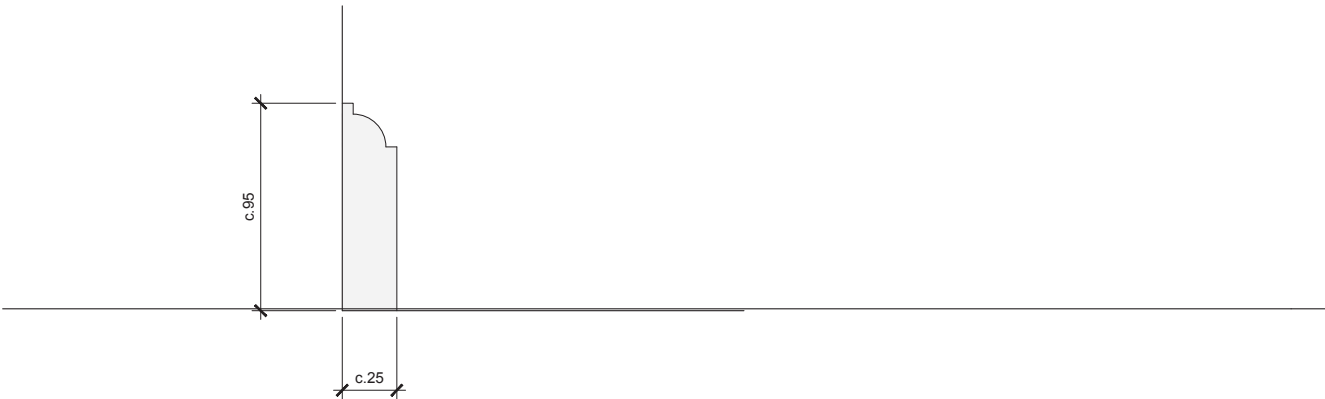
Existing Skirting Section Detail (Dressing Room)
