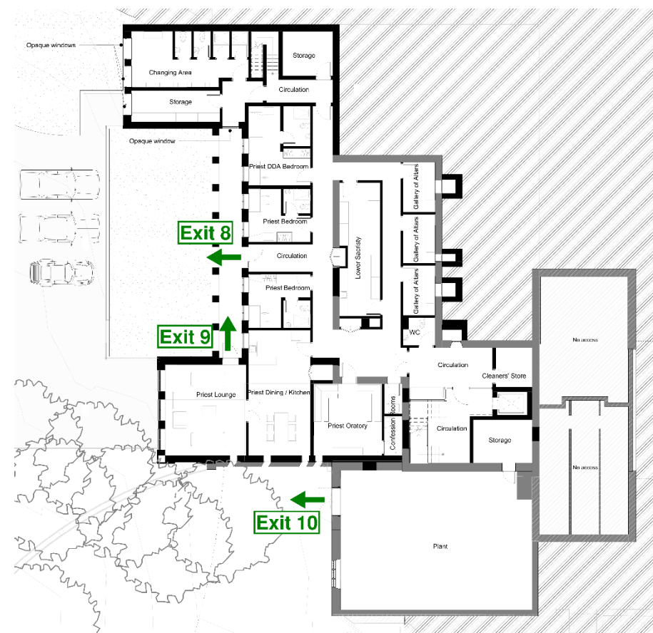
Figure 11 – Manor Building's final exits on the Lower Ground Floor
