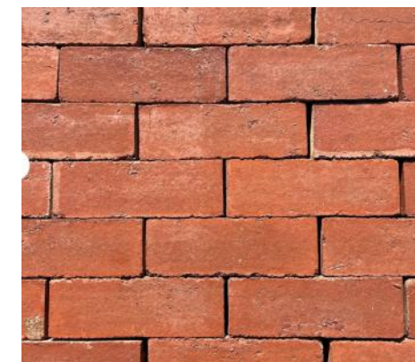
Red reclaimed bricks to match existing.
