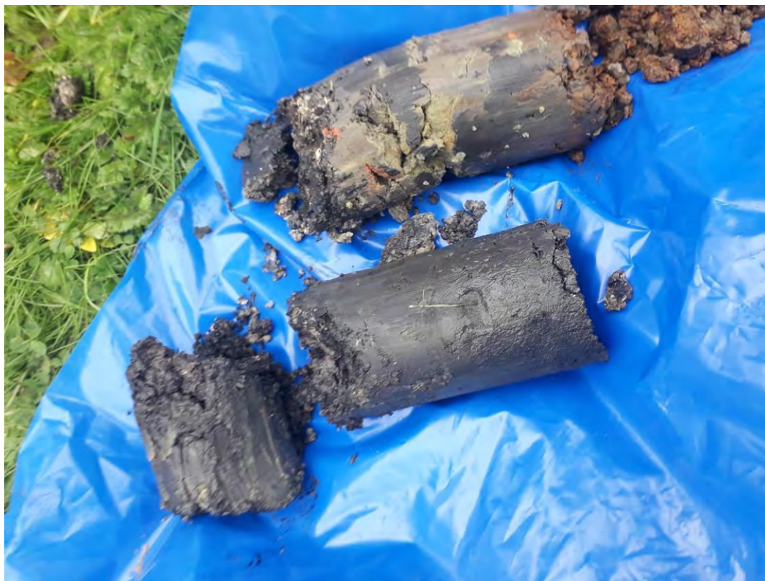
Photograph 6: Photograph of the organic made ground materials encountered within WS2.
