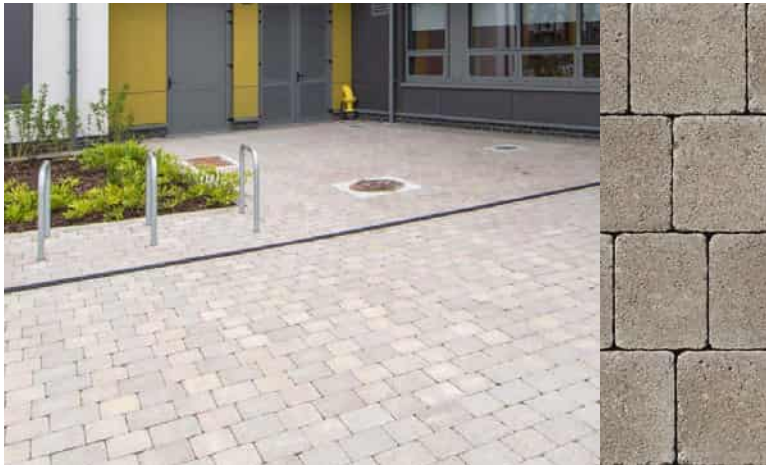
■ Tegula concrete block paving in a three-size mix, 80mm thickness. Colour: Natural. Laid: Stretcher bond. Location: Footpath and pedestrian areas
