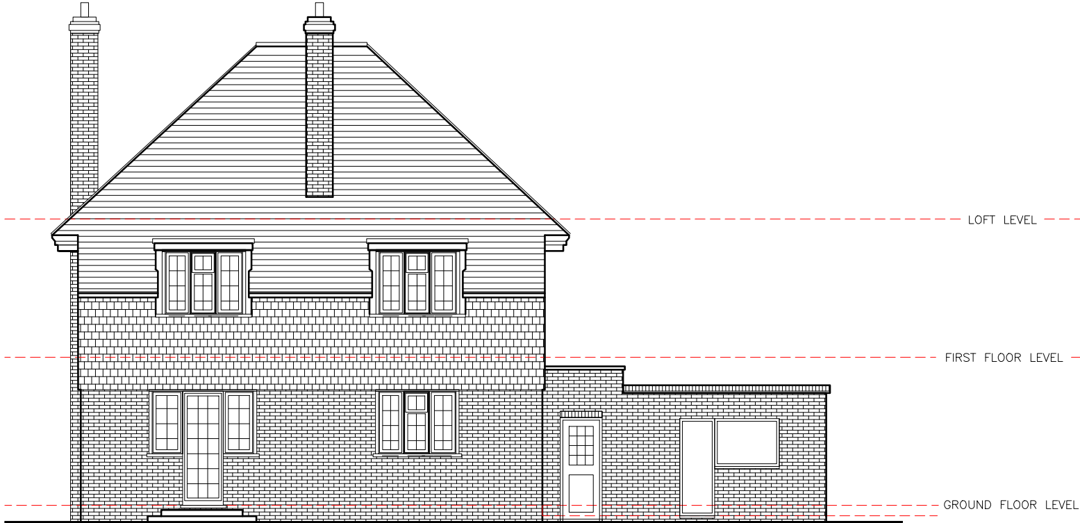
C) Existing Rear Elevation
