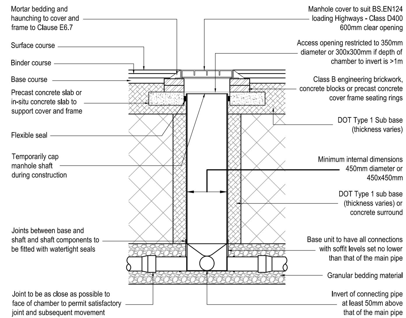
Typical Inspection Chamber Detail - Type D
