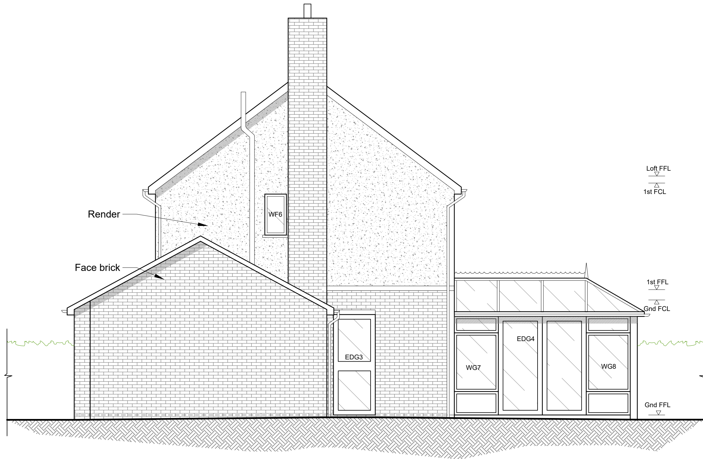
NORTH EAST (SIDE) ELEVATION AS EXISTING
