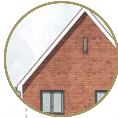
Fascia and gable vent window detail
