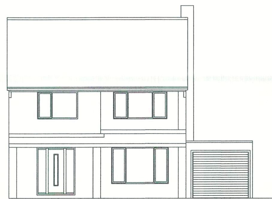
EXISTING FRONT WESTERN ELEVATION 1:100 @ A1.
