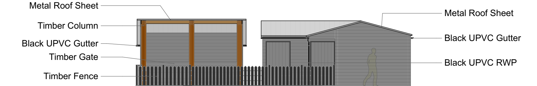
Existing South Elevation
