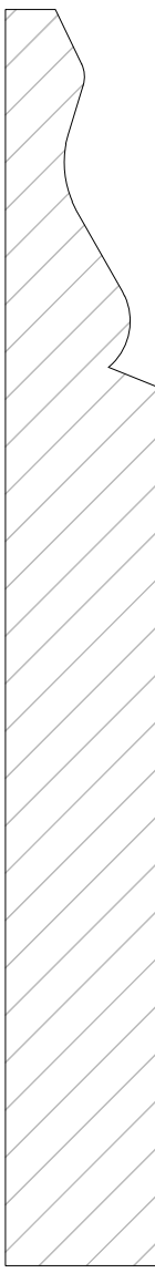
08-Joinery Detail 1:1 Skirting Board
