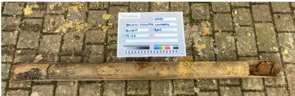
P11: Core run from BH02 between 1.2m and 2.5m depth.
