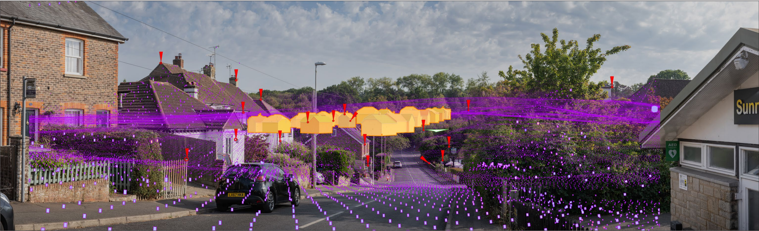
Example composited view demonstrating layers of image data: camera match, photography, digital model and survey/LIDAR data. Red: Bespoke viewpoint survey and alignment. Pink: Supporting LIDAR point cloud. Orange: model of proposed development.
