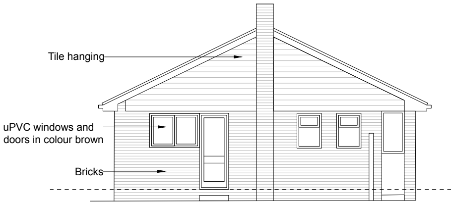
Side (East) Elevation as existing
