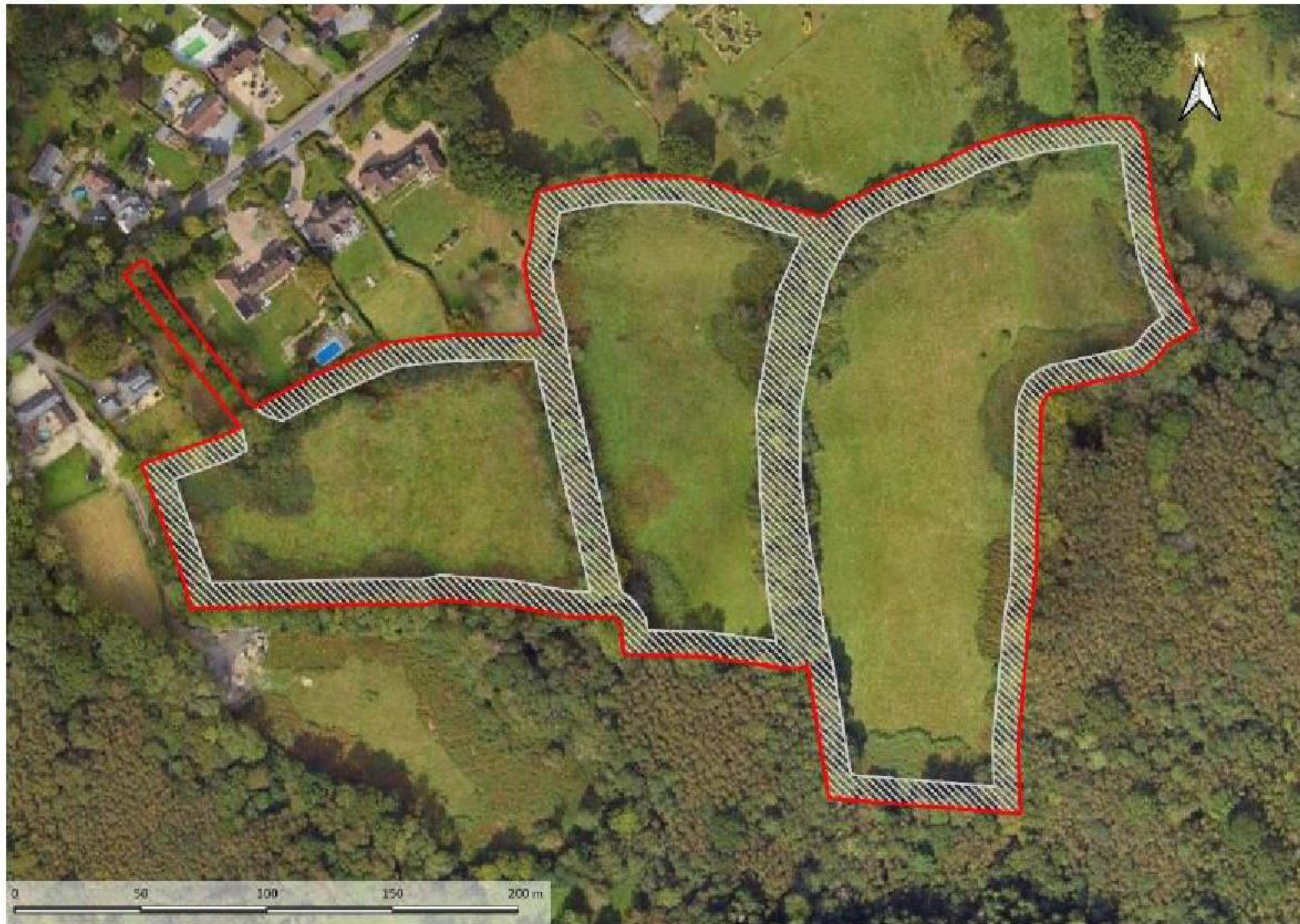
Figure 27. The location of the dark corridors to be implemented into the development, indicated by grey hashing. Light levels in these areas will remain below 0.1 lux.
