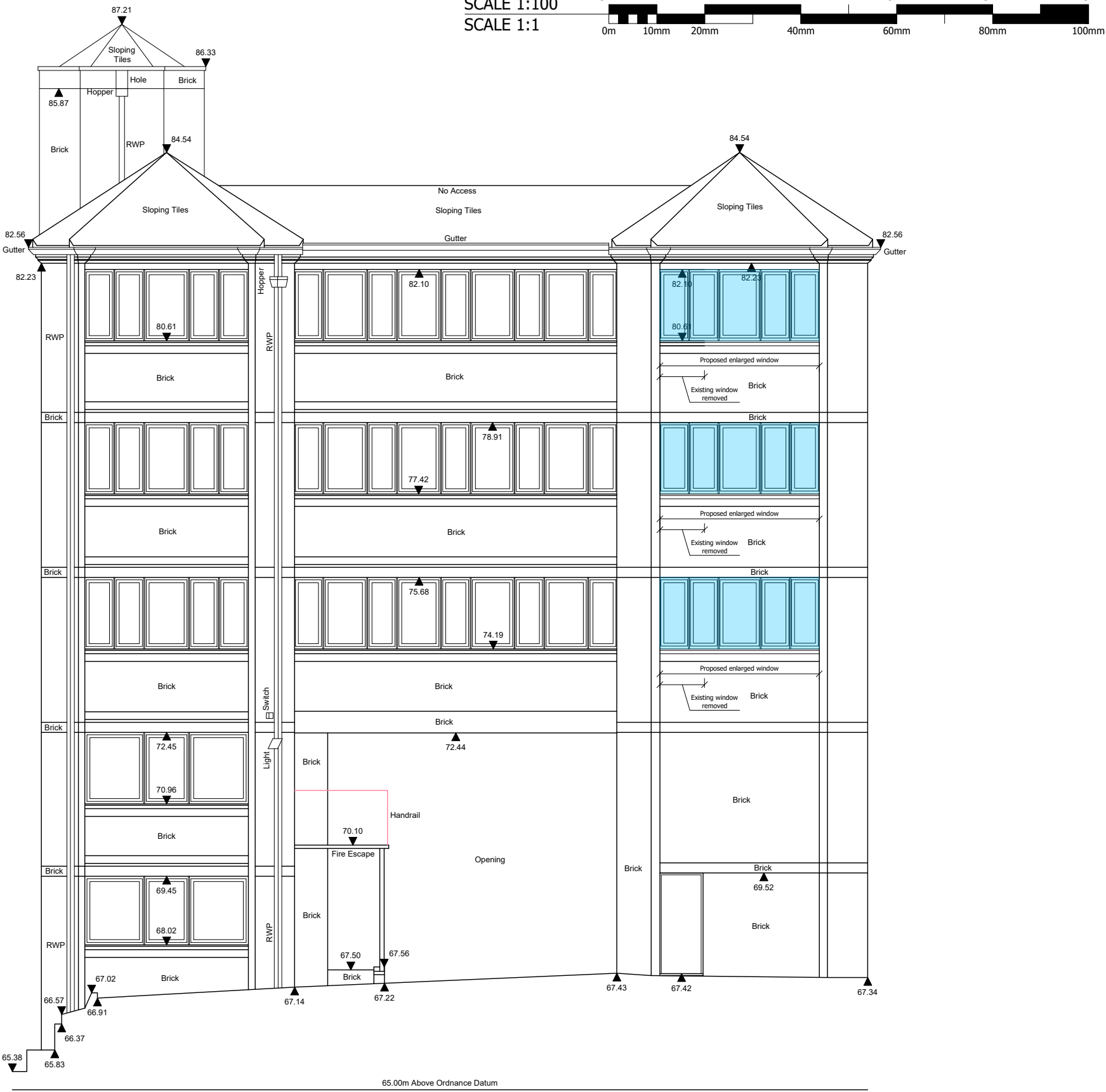
04 West Rear Elevation (3 new windows) Scale 1:100
