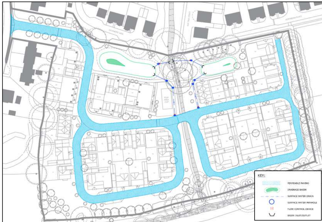
Figure 8.1 - Indicative drainage layout plan showing the proposed location of SuDS.
