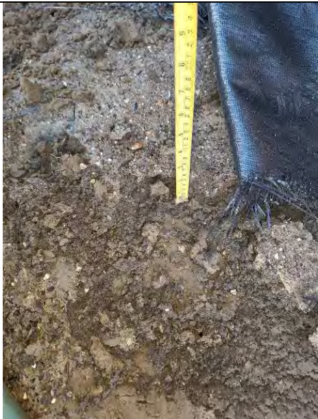
Plate 6: Spot Pit 2, depth of topsoil provided (0.05m).
