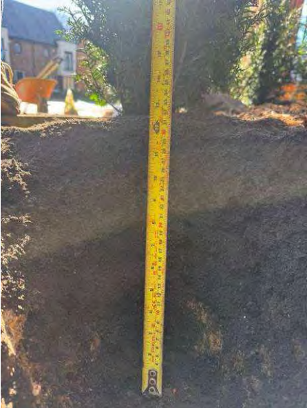
Plate 18: Topsoil placed in the soft landscaped planted area to the east, approximately 300mm cover (assumed to be topsoil and subsoil material).
