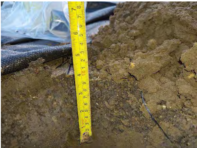
Plate 15: Depth of Topsoil encountered (0.1m).
