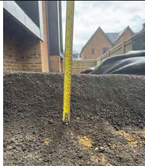
Plate 10: As plates 1, 3, 5 & 8 depth of topsoil provided approximately 0.15m.
