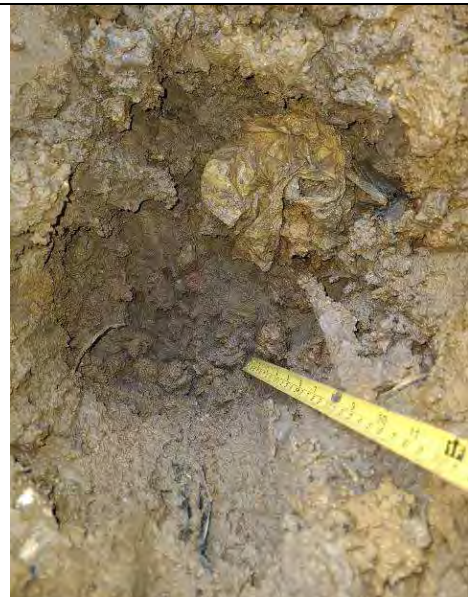
Plate 28: Spot Pit 6, shallow layer of sand Subsoil (0.2m) over silty gravelly CLAY (MADE GROUND) with occasional brick and breeze block pieces.
