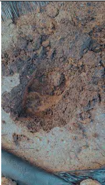
Plate 11: Subsoil encountered in Spot Pit 3 (0.55m). Refusal on stone layer.
