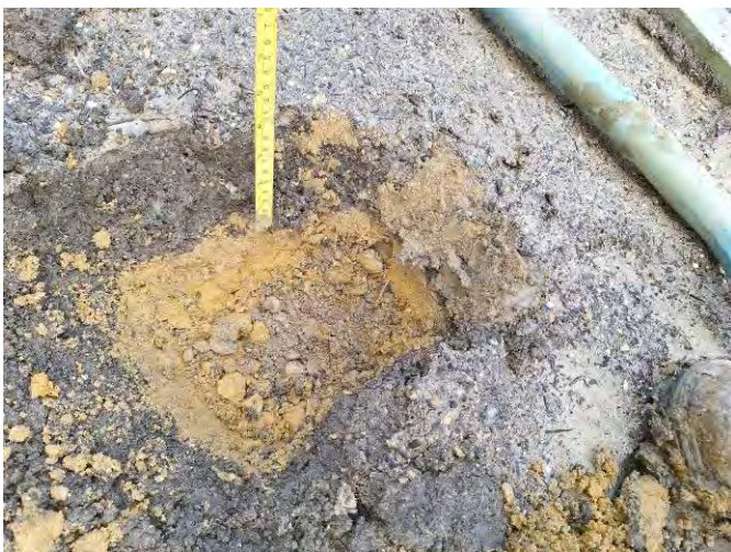
Plate 41: Soils encountered in Spot Pit 8, topsoil placed approximately 0.1m.
