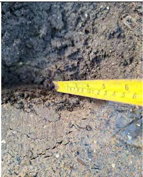
Plate 9: Spot Pit 3m, depth of topsoil provided (0.1m).
