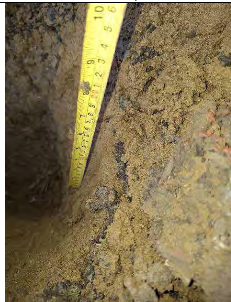
Plate 30: Soils encountered comprised topsoil (0.1m) over silty Sand subsoil (0.18), refusal on stone layer.
