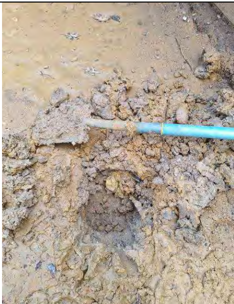
Plate 27: Soils encountered in Spot Pit 6, shallow layer of topsoil (0.05m).
