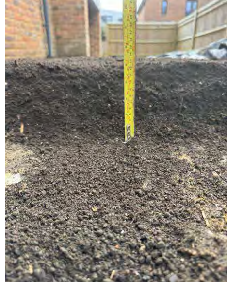
Plate 8: As plates 1, 3 & 5 depth of topsoil provided approximately 0.12-0.13m.
