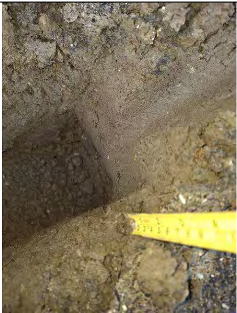
Plate 21: Spot Pit 4, depth of Topsoil (0.1m).
