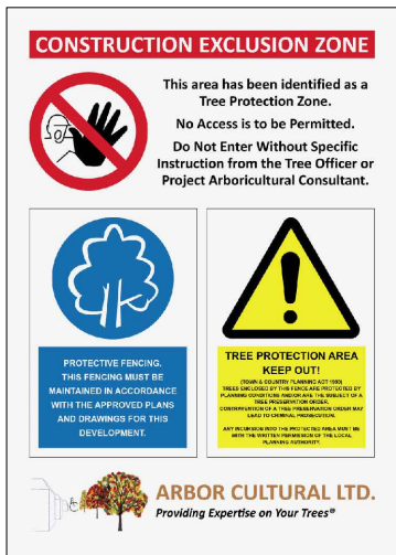
Figure 3 Example of Signage on Fencing
