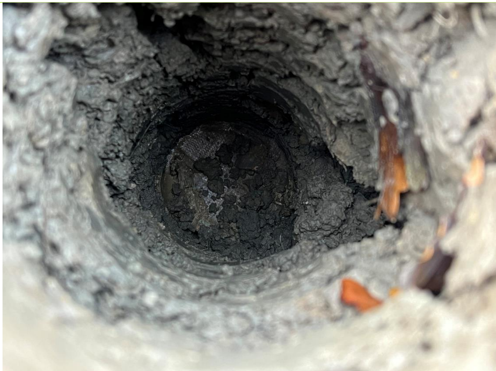
Plate 10 – Overview of Plot 35 rear garden inspection pit showing geotextile membrane at the base of the pit (Dated 21.11.2025)
