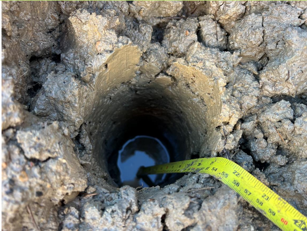
Plate 19 – Plot 3 rear garden clean cover thickness recorded as 550mm (Dated 03.12.2025)
