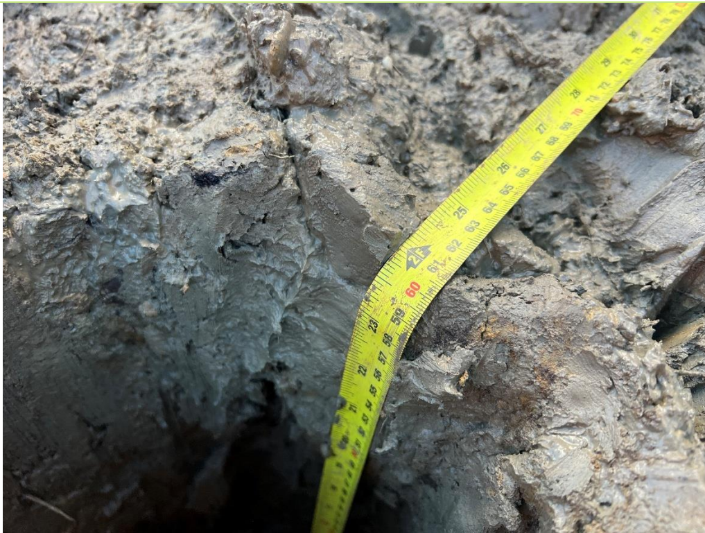
Plate 15 – Plot 5 rear garden clean cover thickness recorded as 600mm (Dated 03.12.2025)
