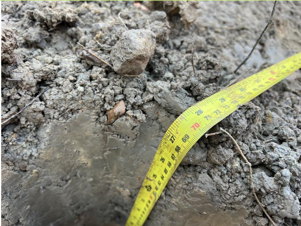
Plate 9 – Plot 35 rear garden clean cover thickness recorded as 700mm (Dated 21.11.2025)
