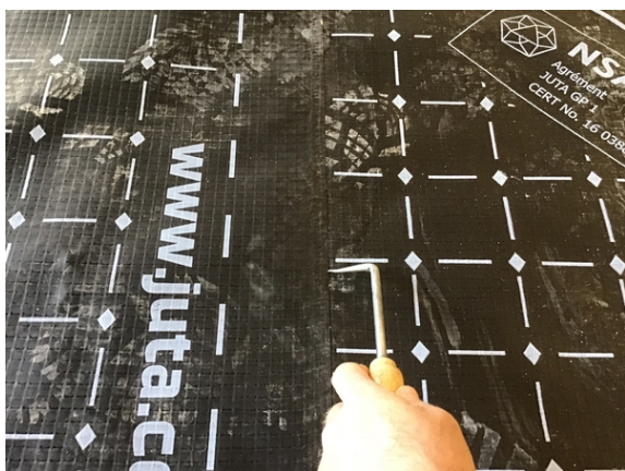
Probe testing a typical hand welded membrane lap in plot 10.
