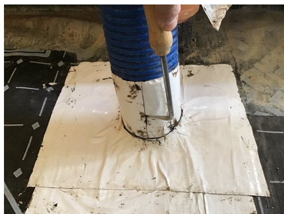
Probe testing a typical pipe penetration detail in plot 9.
