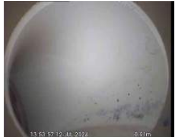
SVPX_1a7c91c5-7811-4395-aac0-3828833b4982_20240725_095342_984.jpg, 00:00:49, 0.91 m Line deviates left
