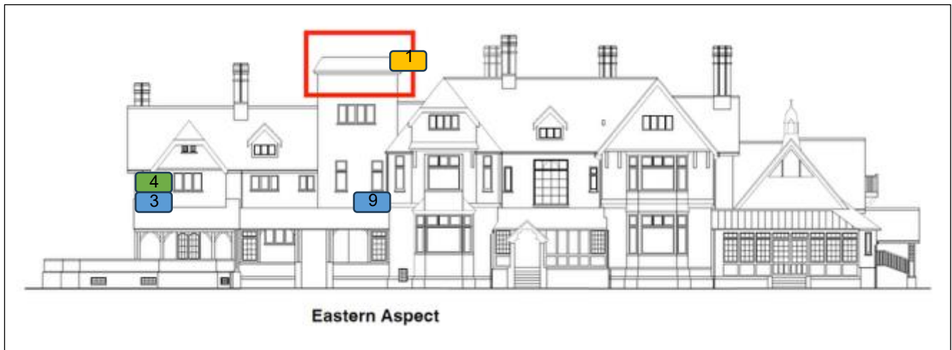
Figure 35. View of the approximate bat roost locations on the eastern aspect with the approximate areas of development indicated in red boxes. Numbered squares indicate roost locations and numbers (Table 2) blue indicating common pipistrelle, green indicating soprano pipistrelle and orange indicating brown long eared bat. Image produced courtesy of Ian Adam Smith Architects.
