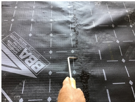
Probe testing a hand welded membrane lap in plot 36.
