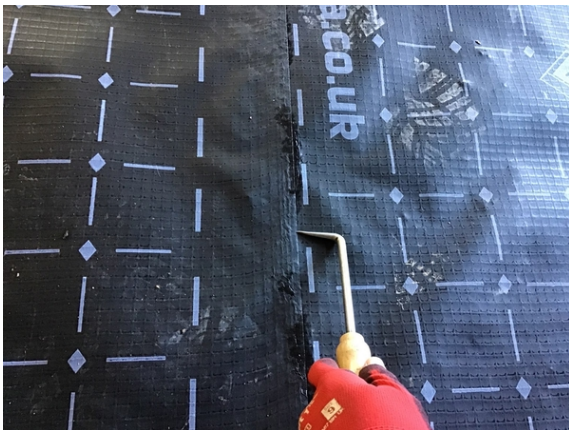
Probe testing a typical hand welded membrane lap in plots 6 & 7.
