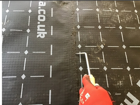
Probe testing a hand welded membrane lap in plot 27.
