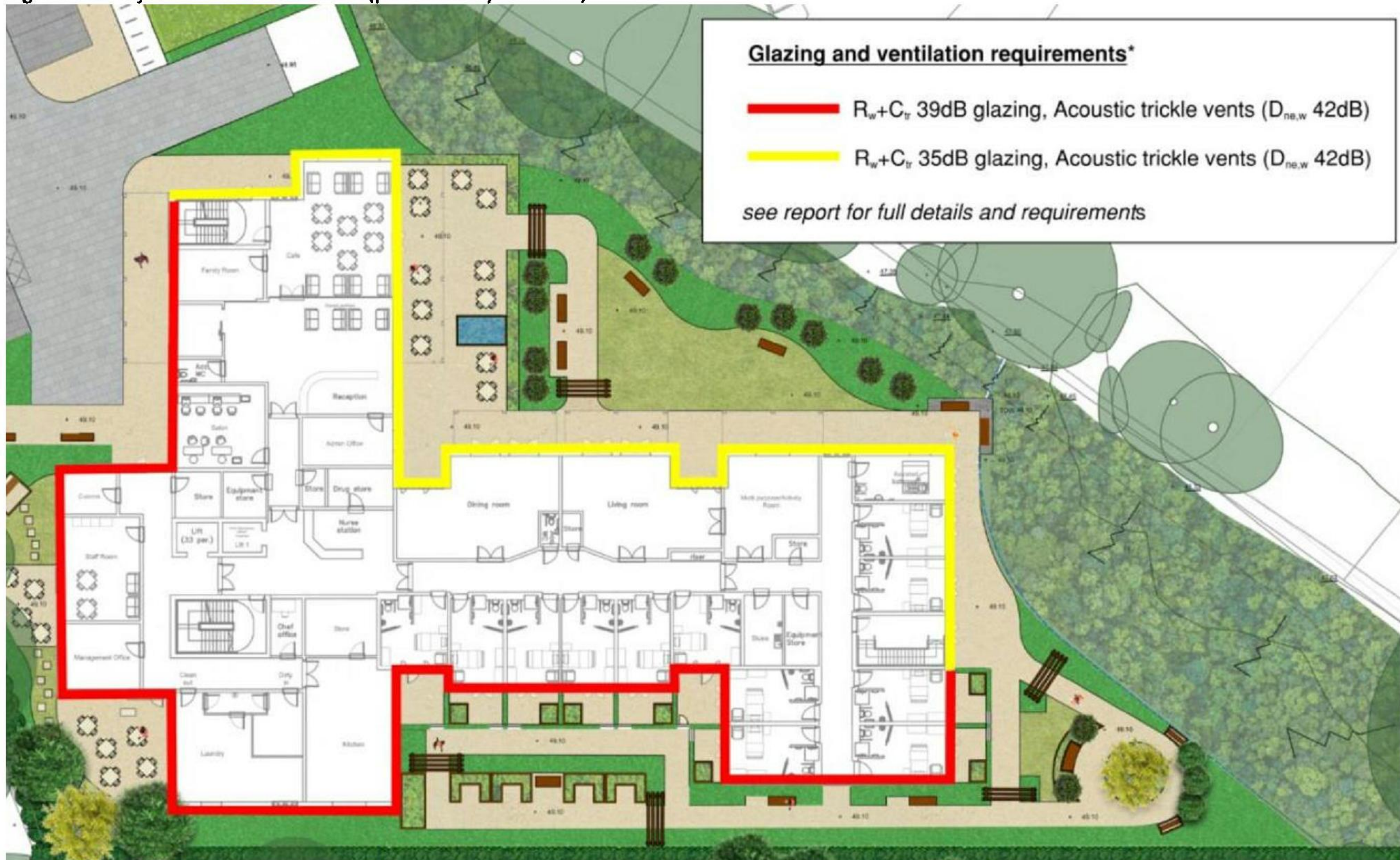
Figure 3-4: Façade Element Locations (produced by Ramboll)
