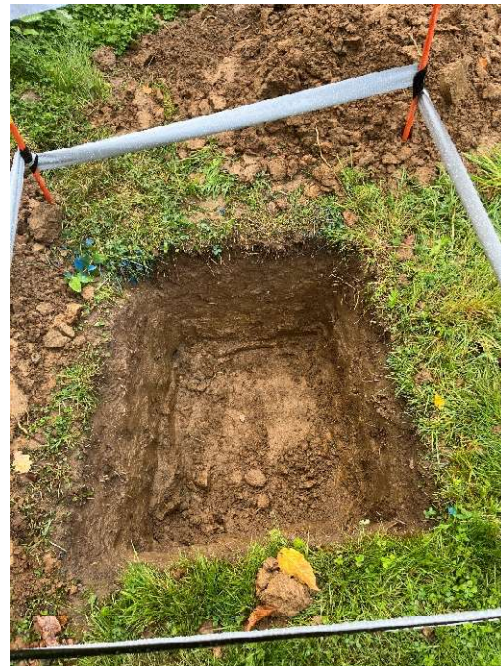
Soakaway Test Pit – 0.9L x 0.8W x 0.6D
