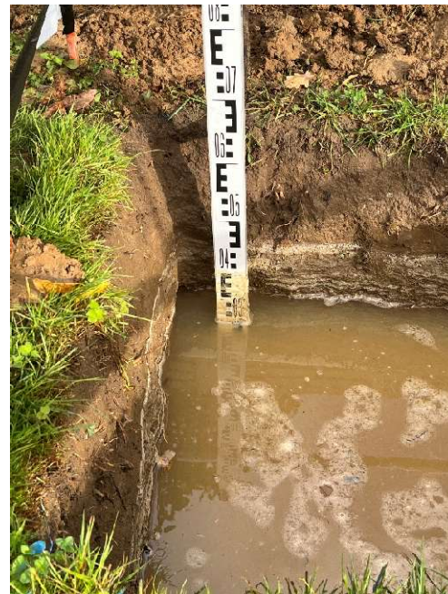
Soakaway Test Pit – Water Level 300mm
