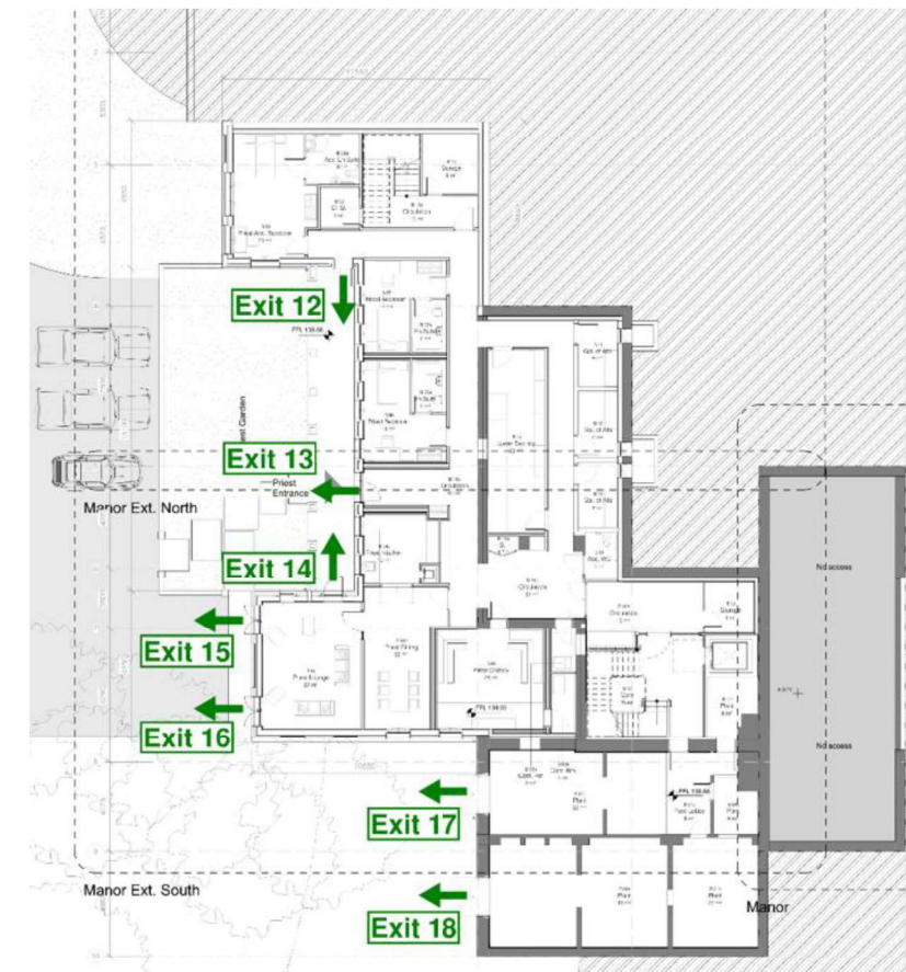
Figure 11 – Manor Building's final exits on the Basement Floor
