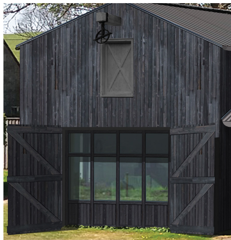
5 Shiplap sweet chestnut gate flushed with wall cladding
