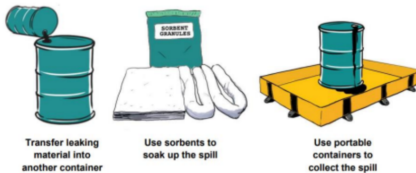
Examples of how to control a spill close to the source
