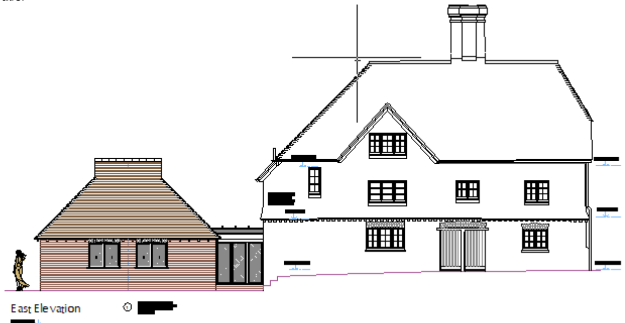
Fig.4: East Elevation showing proposed extension
