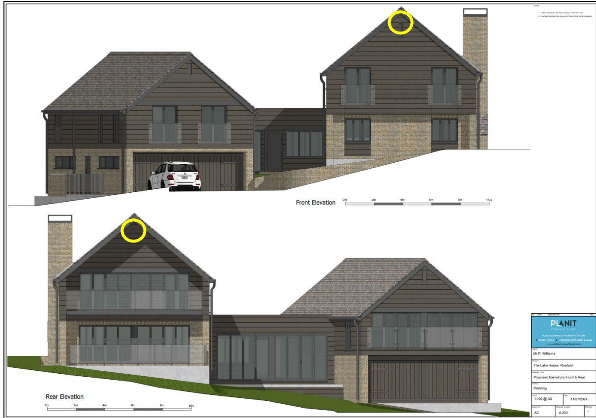
Figure A6.1: Proposed front and rear elevations with suggested bat box locations (yellow circles) (Adapted from Planet Consulting, 11 th July 2024, drawing number: A.203).
