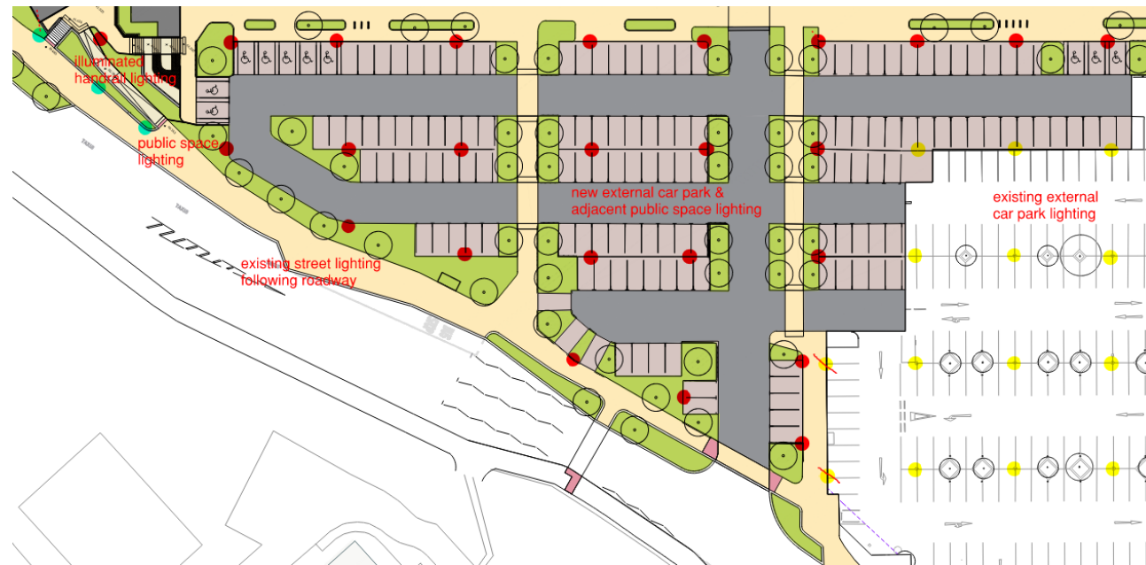
Figure 1 - New External Car Park Lighting Area
