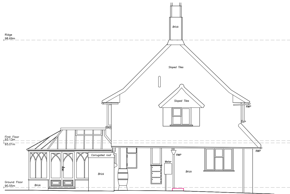
02-Side Elevation (south) 1:100 Existing
