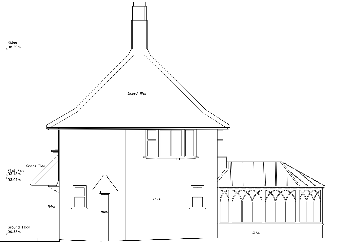
04-Side Elevation (north) 1:100 Existing
