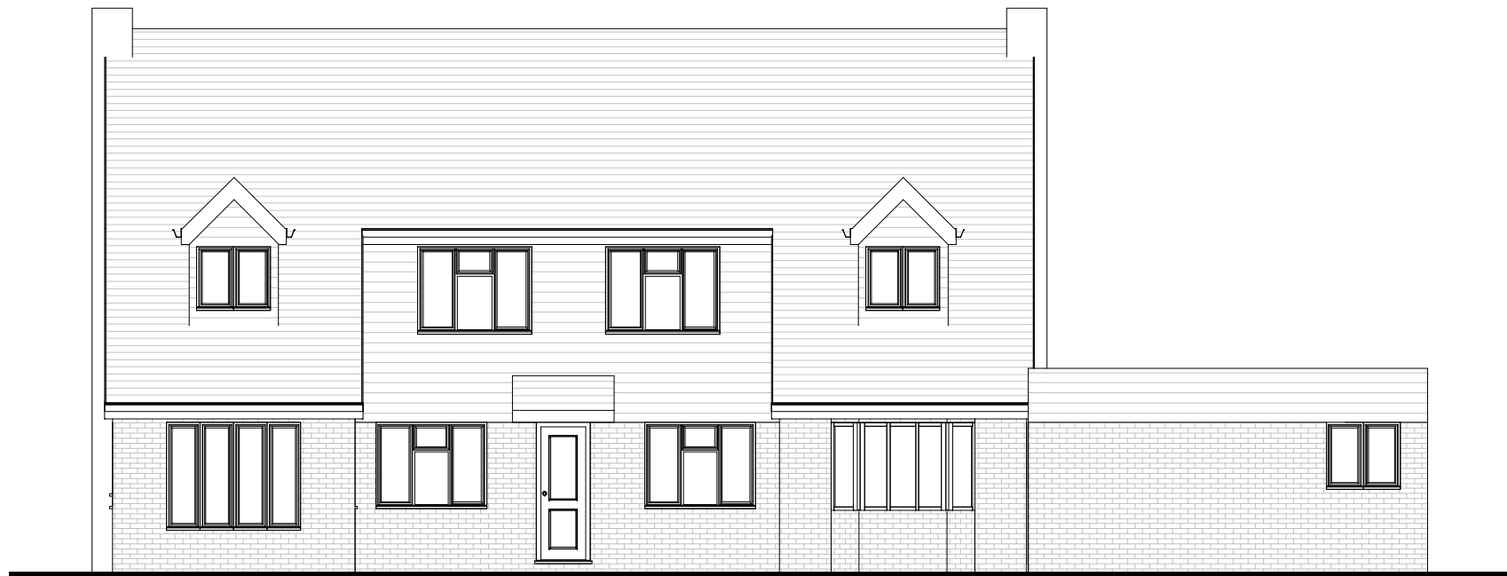
Front Elevation - Existing - 1:100
