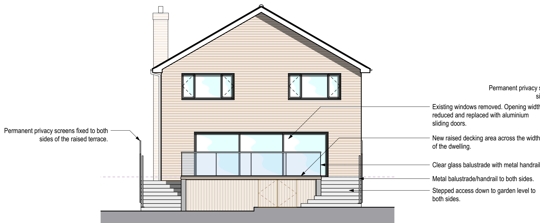
E3 REAR ELEVATION - South Scale: 1:100
