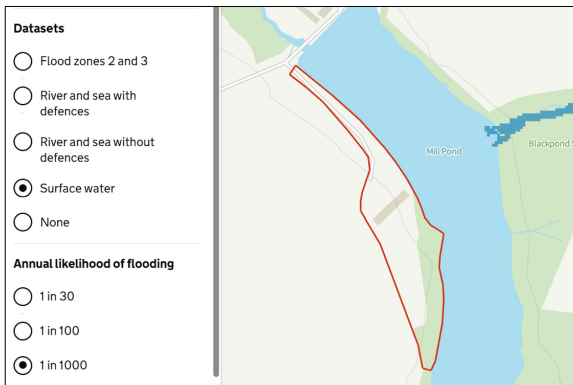
Figure 4.1 – 1 in 1,000-year Surface Water Flood Risk Extents
